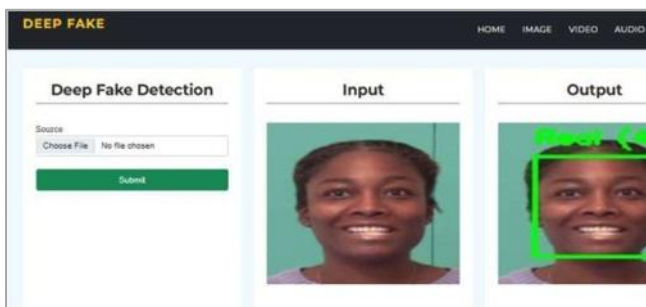
Fig. 2. Detection of a real image. The face region was localized with MTCNN, processed by a ResNet-50 backbone, and classified as Real with a high confidence score.
