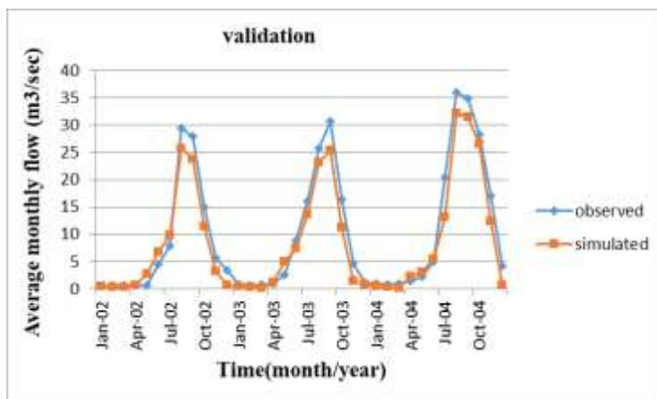
Figure 15: Comparison of observed and simulated discharge for the validated model.
