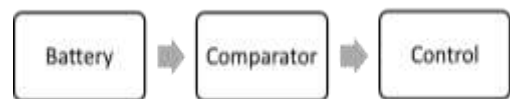
Figure 1: Block diagram for load shedding battery cut-off circuit for solar powered system
