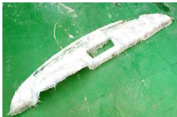
Figure 2. Cope molds for manufacturing of PEUGEOT model vehicle dashboard.
