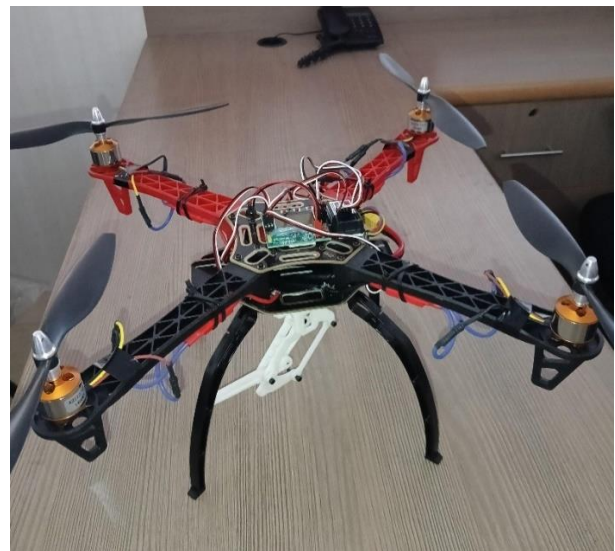
Figure 5: Drone with 3-DOF arm
